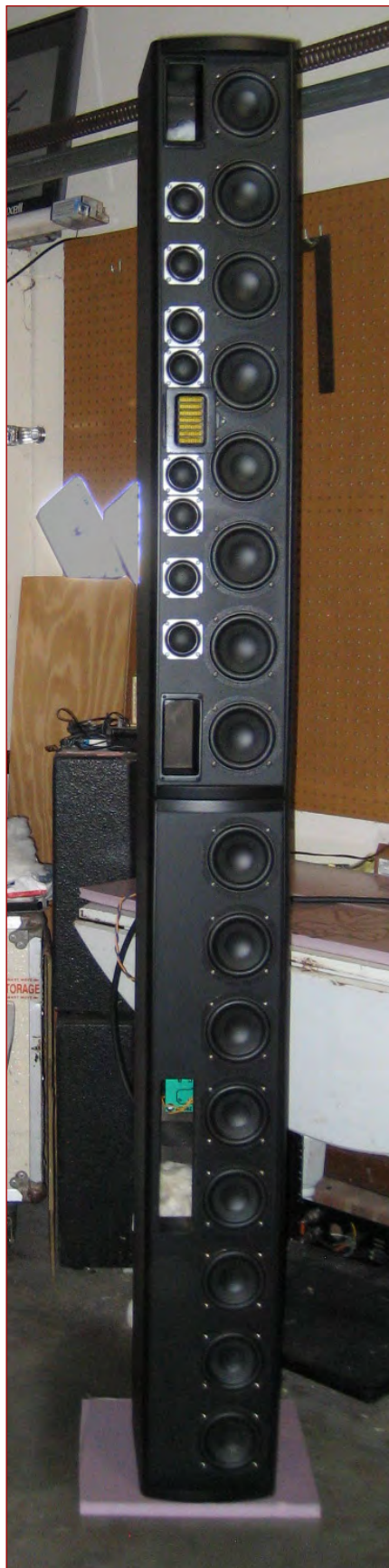
Charlie recently finished designing a speaker for SoundTube. The speaker features a line-array point source (LAPS) design.
