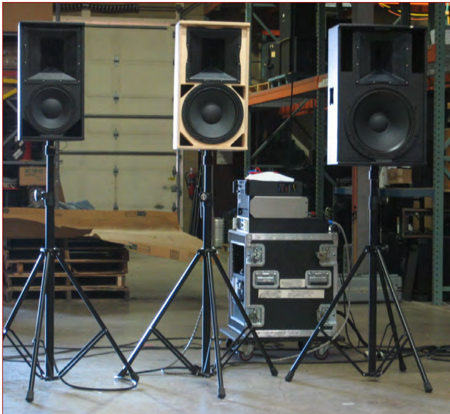
Charlie recently designed three two-way loudspeakers for Bag End. Each has a 10", 12", and 15" woofer.
