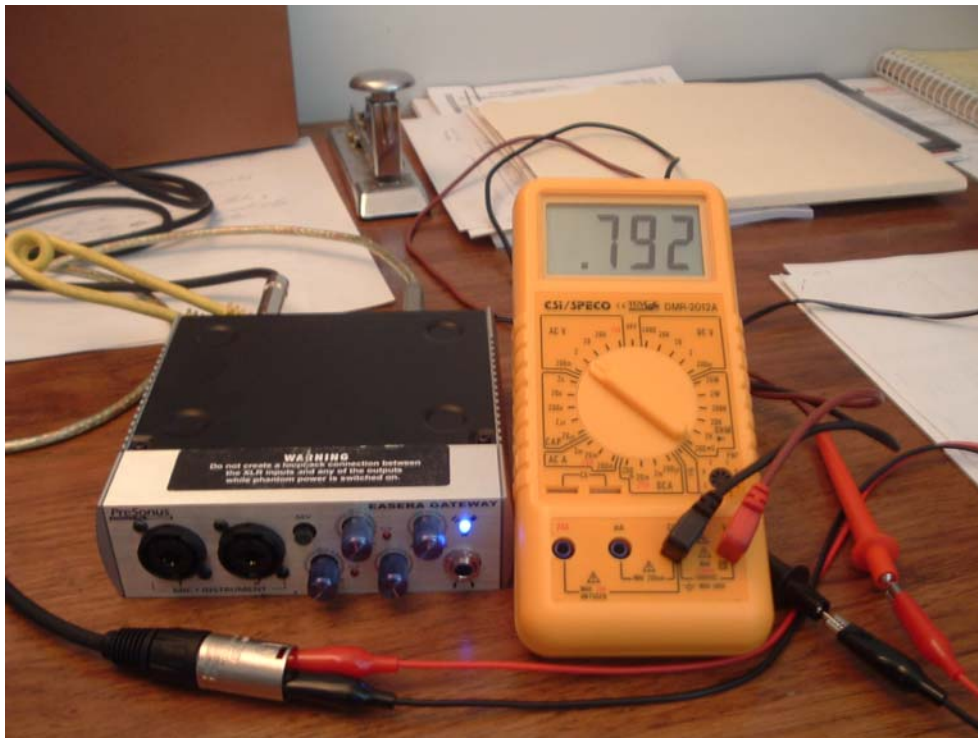
Figure 6 – RMS voltage at 1 kHz measured with a digital multi-meter
