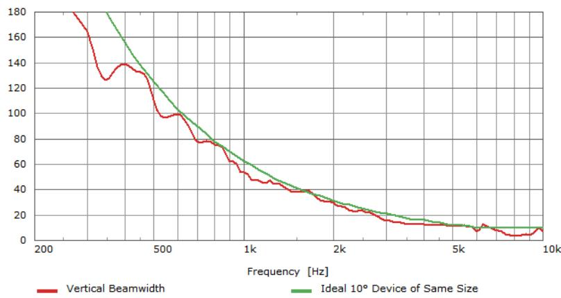
Figure 14: Vertical beamwidth of dual PDE prototype (red) and theoretical ideal 10° of the same size (green)
