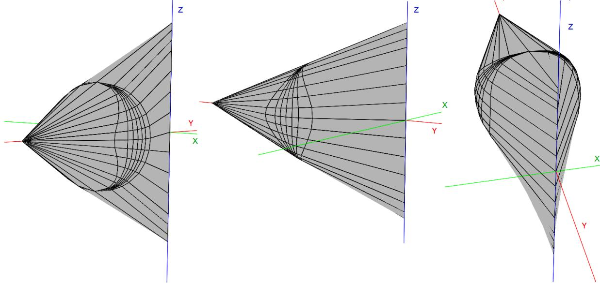
Figure 5: Shape of an inner core for a phase plug
