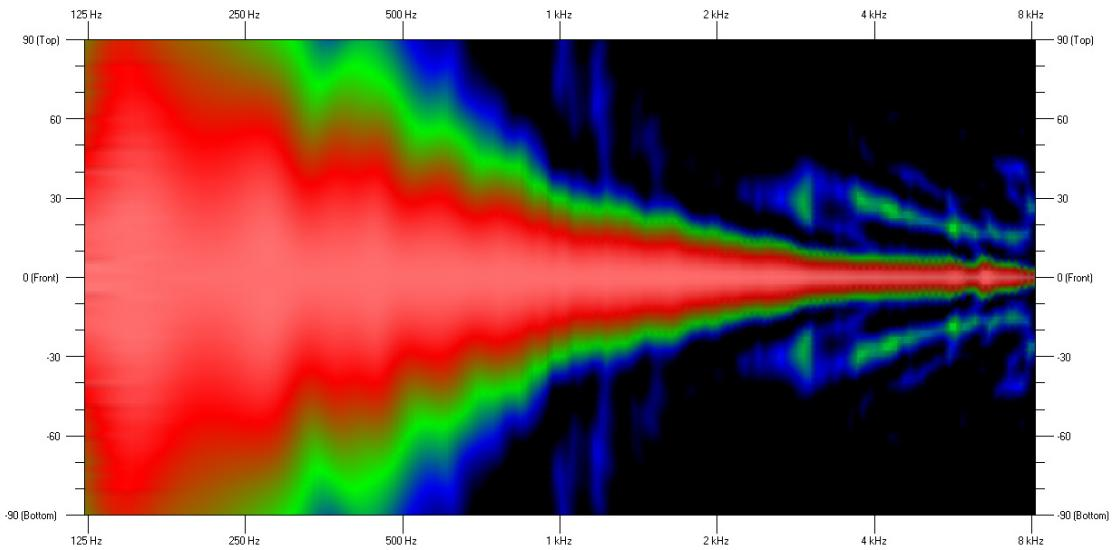
Figure 15: Vertical directivity map of dual PDE prototype device
