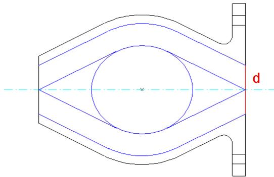
Figure 7: Top view of phase plug showing offset distance from the inner core to define the outer shell
