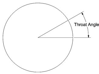
Figure 9: Throat Angle for the Outer Core
