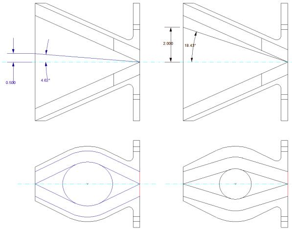
Figure 2: Two different angular cross sections (upper) and the normal projection to each of the angular cross sections (lower)
