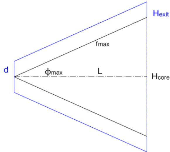
Figure 3: Side view of basic phase plug geometry
