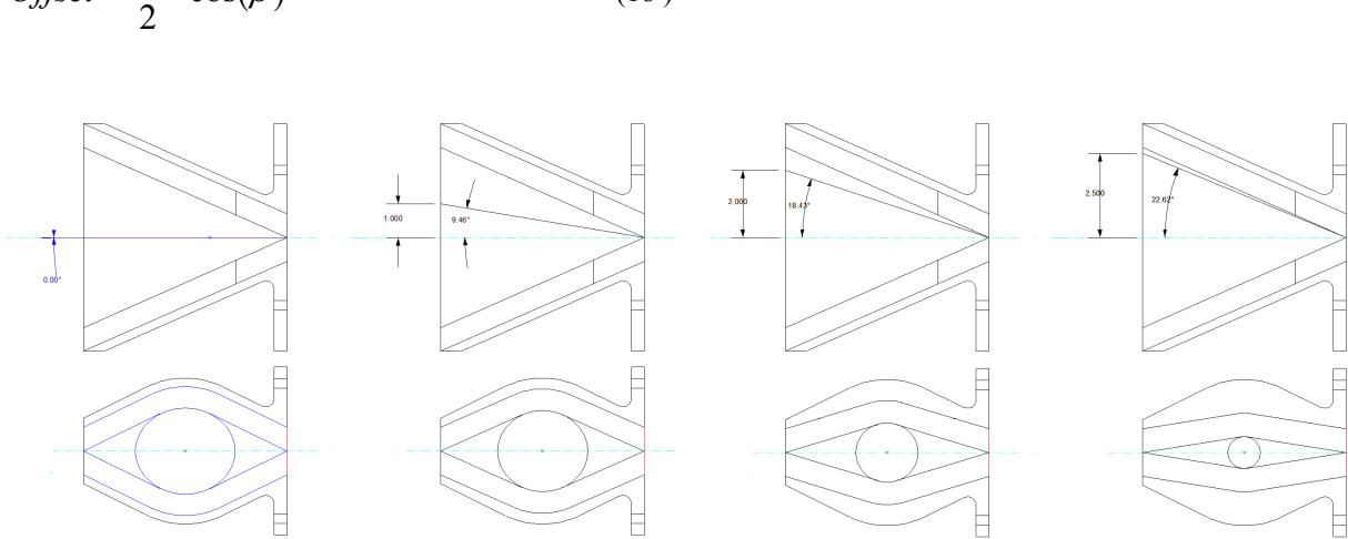
Figure 8: Different cross sections,  $\varphi$ , through the phase plug
