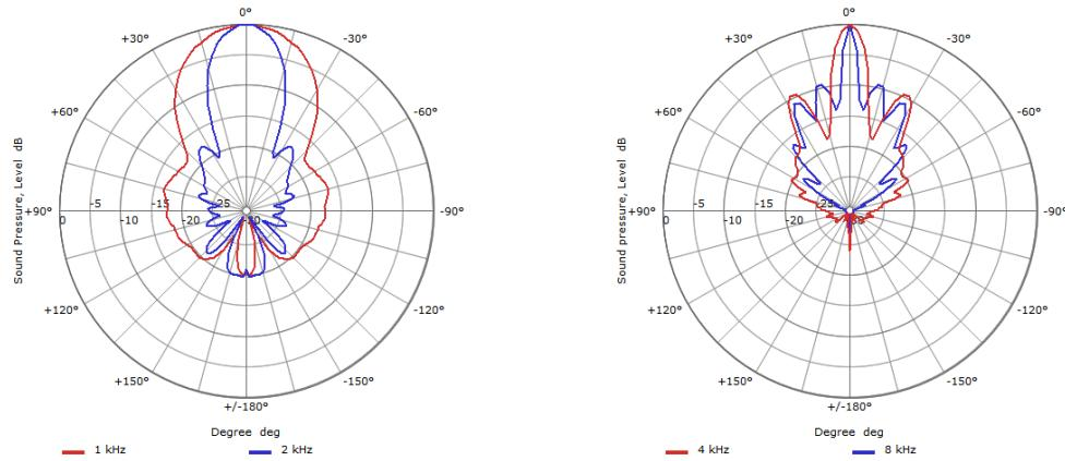
Figure 13: Vertical polar plots for dual PDE prototype at 1 kHz, 2 kHz, 4 kHz, and 8 kHz
