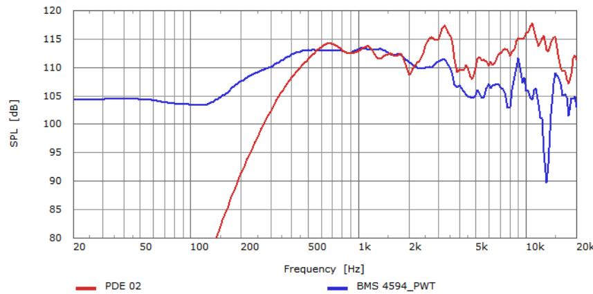
Figure 12: On-axis response of dual PDE prototype (red) and compression driver on plane wave tube (blue)
