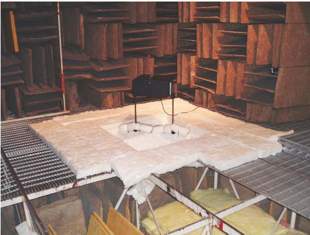
Photo 7 – Absorption on non-removable floor grates and in the well housing the turntable
