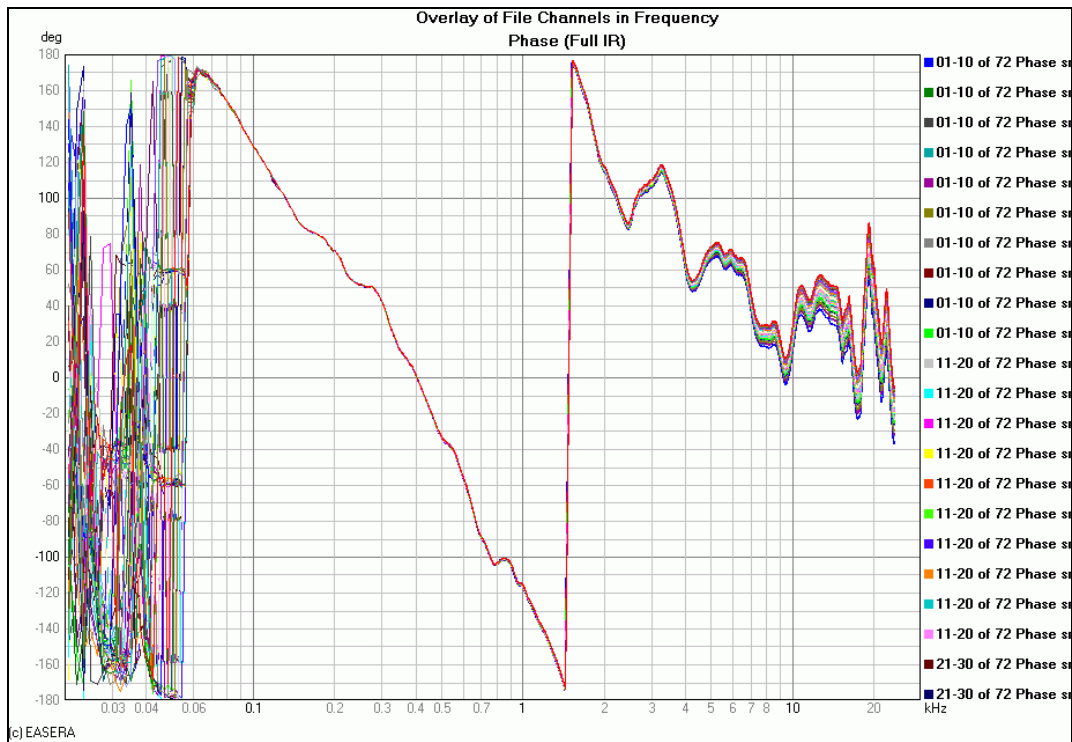
Figure 4 – 72 different phase response curves of the 0° mic for the front hemisphere of a balloon (Note that at 13 kHz all of the curves are within 20° of each other, most of them are within 10°)
