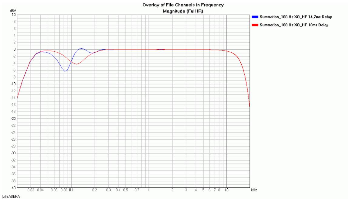
Figure 5 – Magnitude response summed response with the cluster delayed 10 ms (red) and 14.7 ms (blue)
