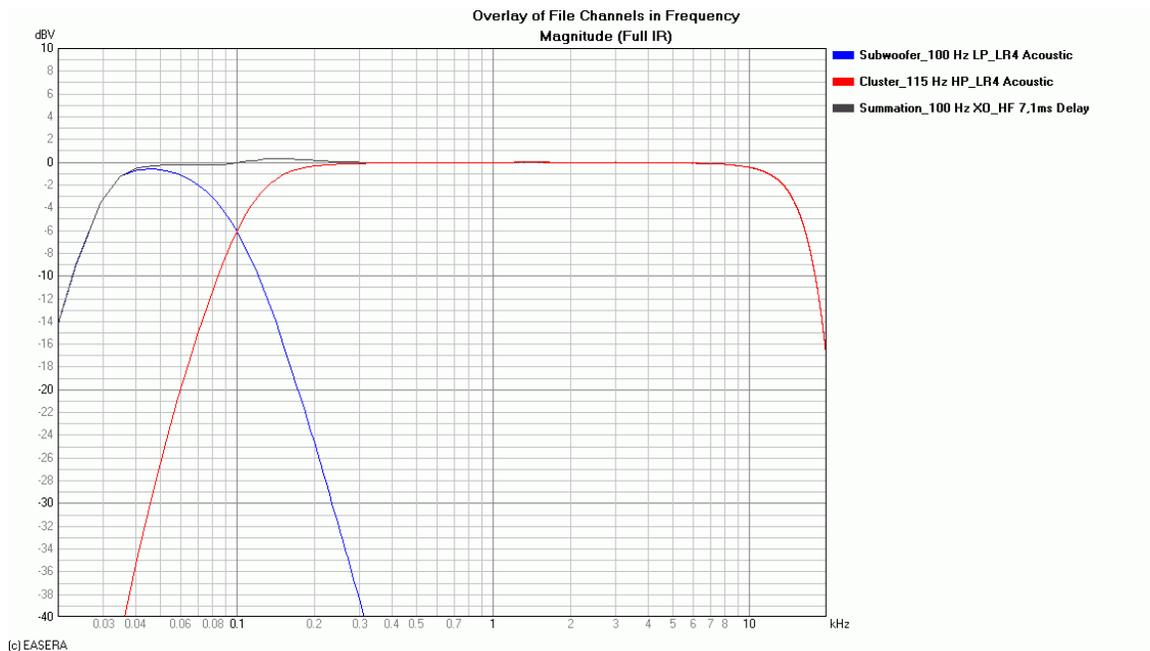
**Figure 8 – Magnitude response of individual pass bands and the summed response with the cluster delayed 7.1 ms**
